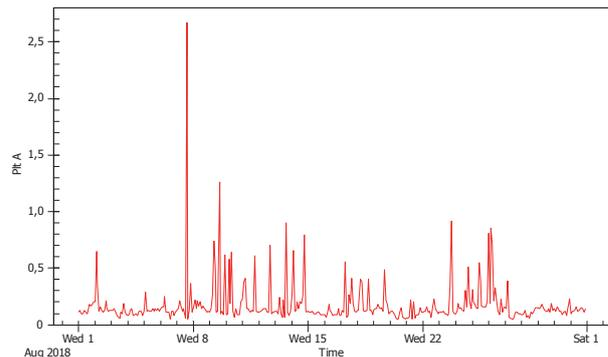
Figure 4. Long term flicker at 400 kV transmission line during breakdown
