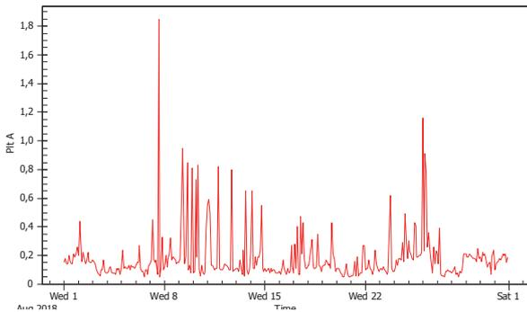
Figure 6. Long term flicker at 110 kV lines after 400 kV lines breakdown
