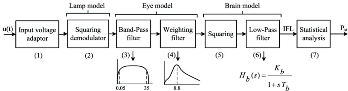
Figure 2. Block diagram of a standard IEC flickermeter [11]
