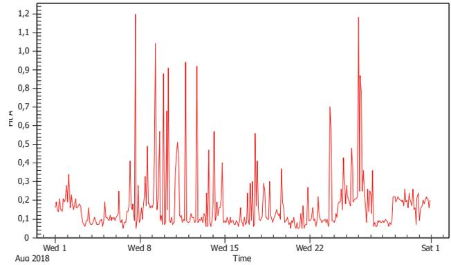
Figure 9. Long term flicker at 110 kV substation TS D, after 400 kV lines breakdown
